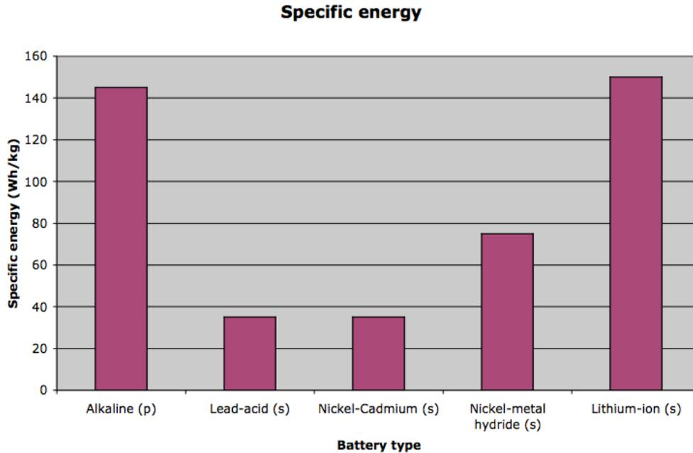
**Figure 6: Alkaline and Lithium-ion batteries are superior choices for robotics applications due to their high specific energy**
