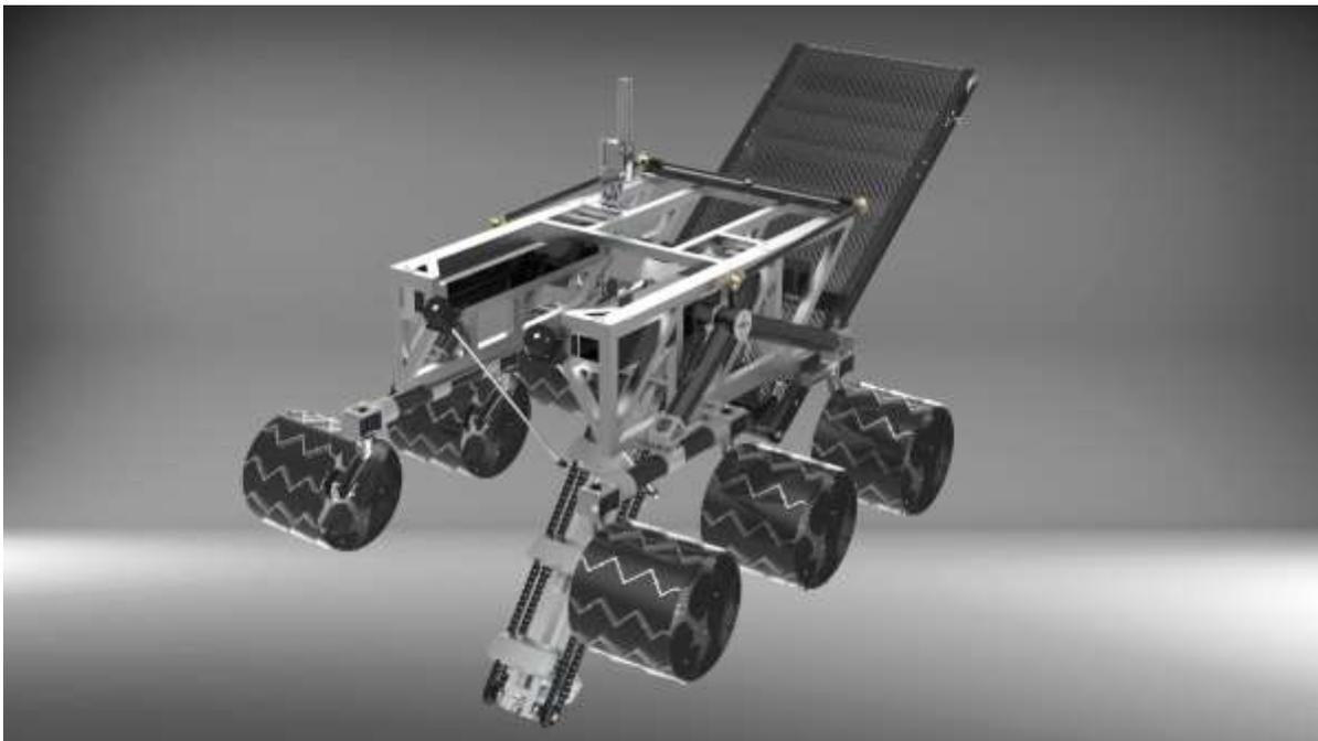
**Figure 5: UP Rover CAD in a fully “Unpacked” State**
