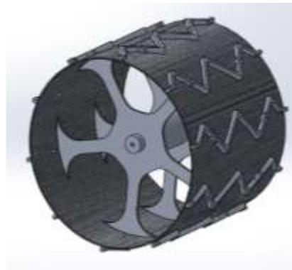
**Figure 3: Hybrid wheel alternative.**
