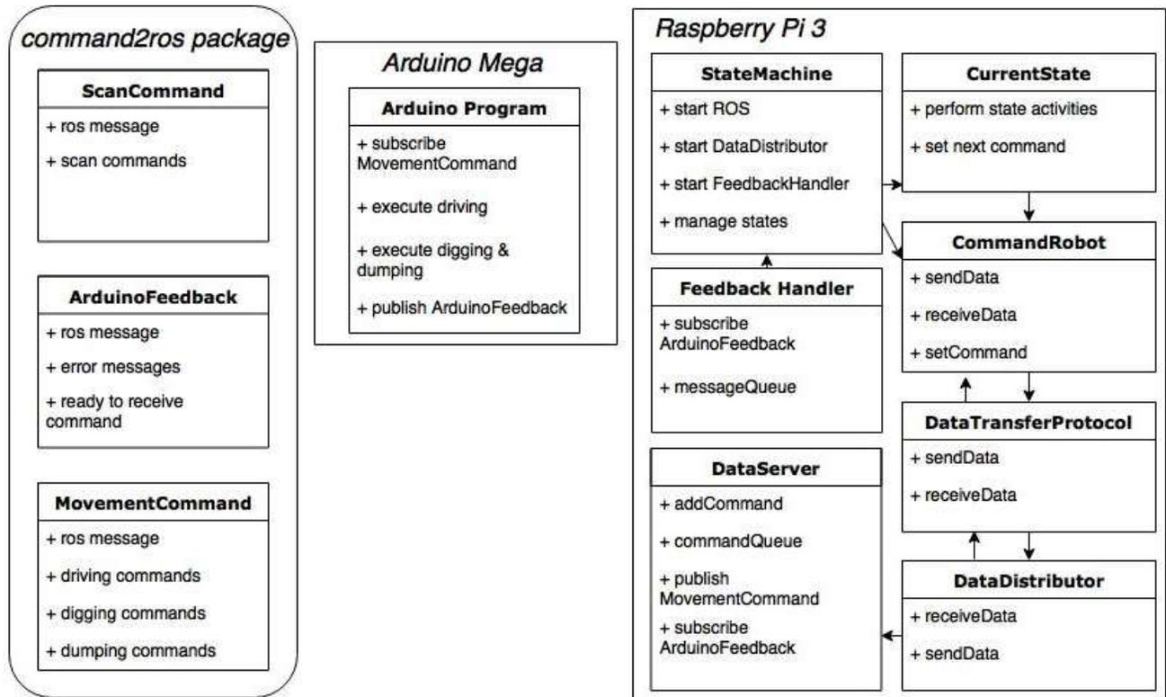
Figure 8: Software System Communications
