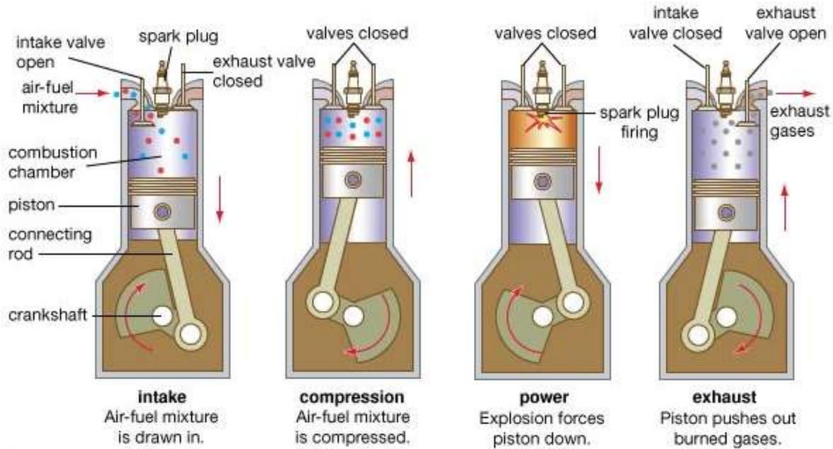
Figure 2: Operation of the four-stroke engine cycle<sup>3</sup>
