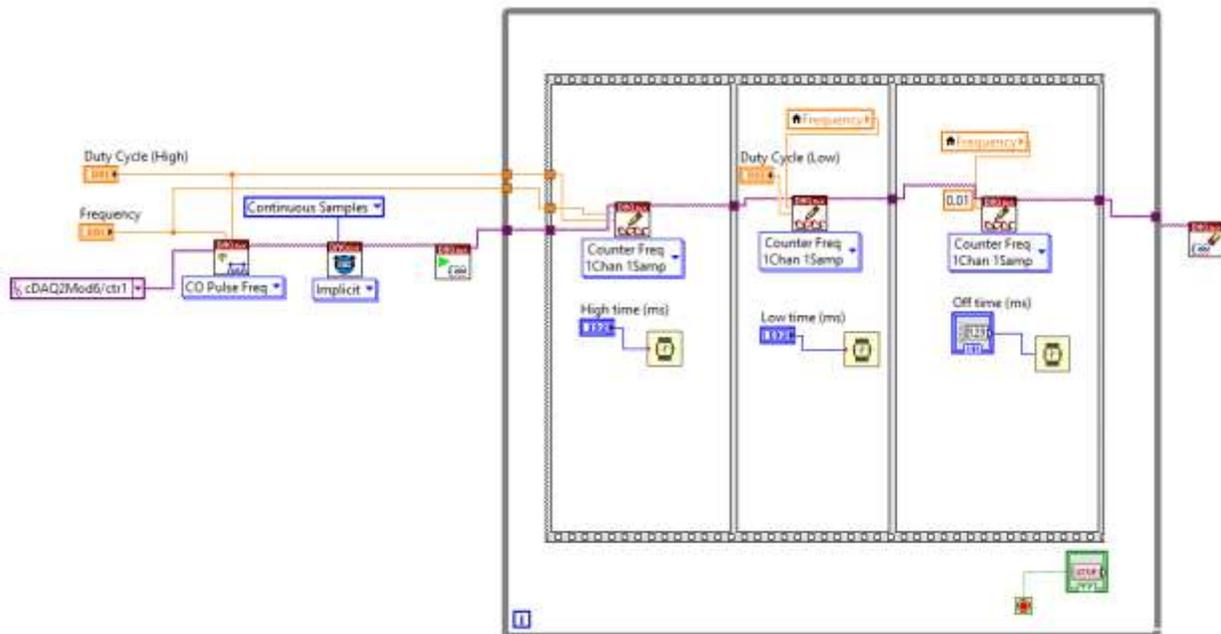
Figure 13: Prototype LabVIEW Control System Block Diagram
