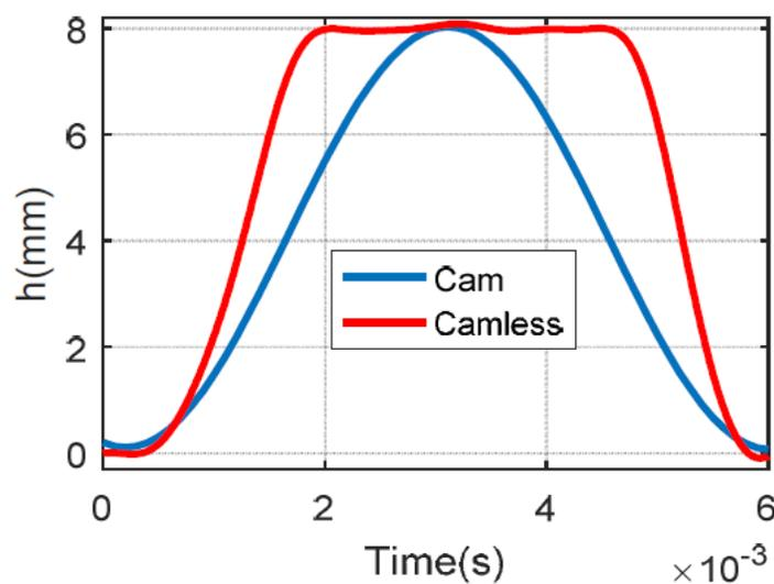
Figure 4: Comparison of Valve Position in Cam and Cam-less Systems<sup>6</sup>
