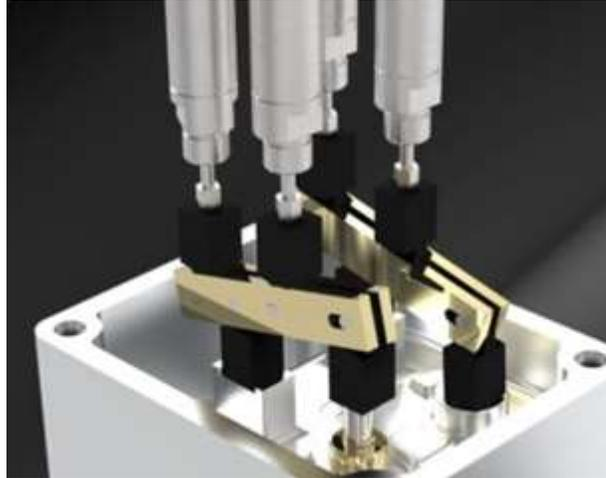
Figure 15: Model of Rocker Valve Actuation System
