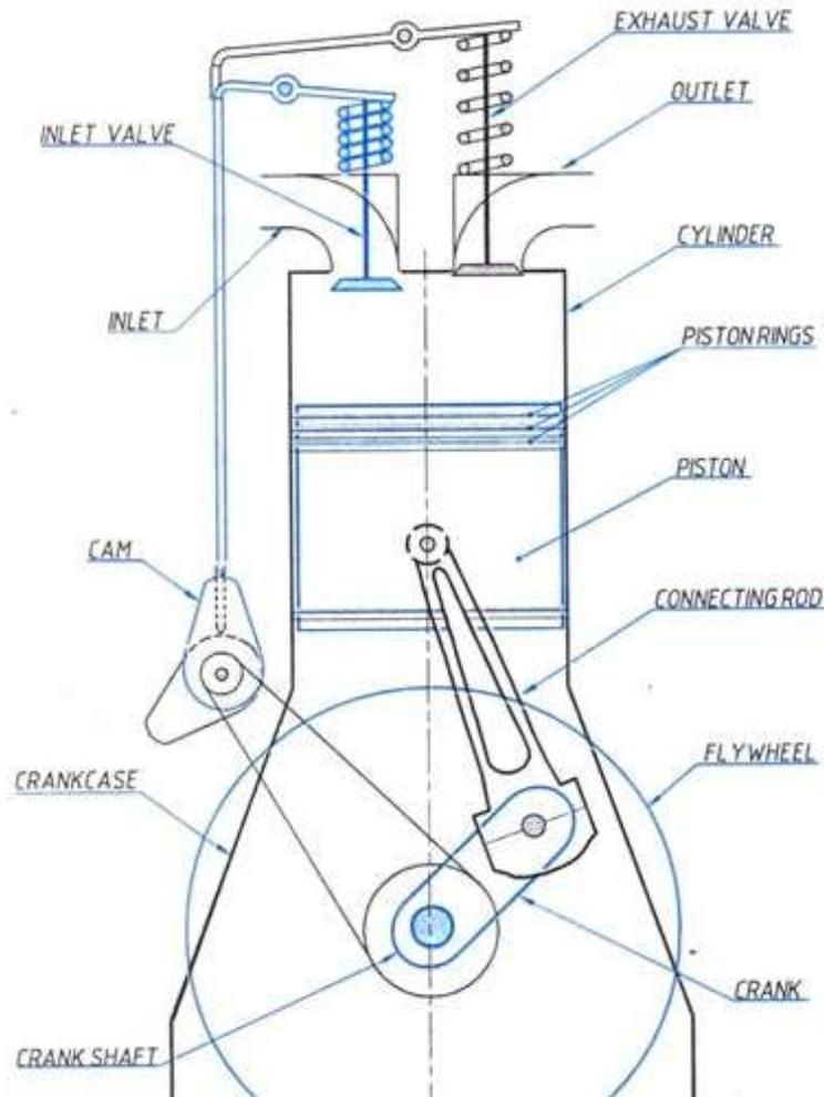
Figure 1: Cutaway Diagram of Internal Combustion Engine Cylinder<sup>2</sup>
