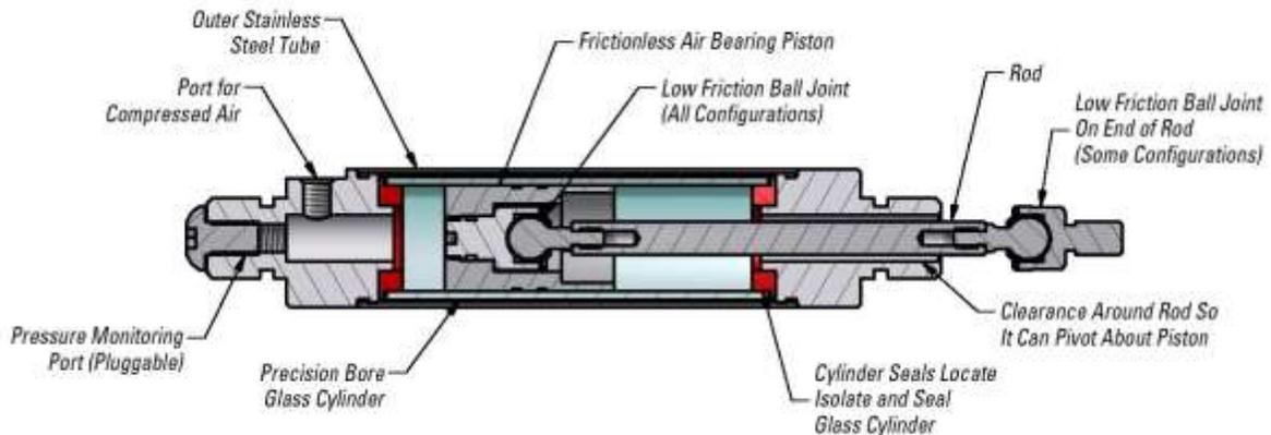
Figure 11: Airpot Corporation Airpel AB Pneumatic Ram Schematic <sup>15</sup>
