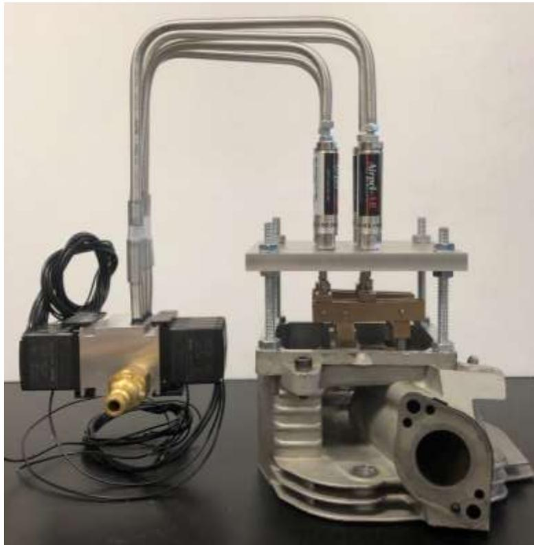
Figure 16: Final Valve Actuation System Assembly
