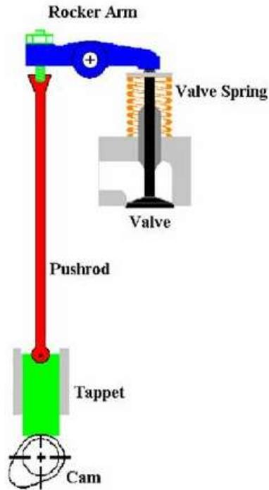
Figure 3:Components of the Camshaft-Based Valvetrain<sup>4</sup>
