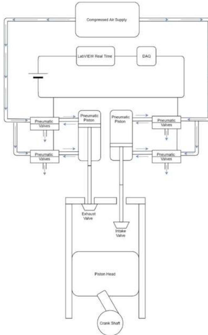
Figure 7: Initial Design of Pneumatically-Actuated Electromechanical Valvetrain
