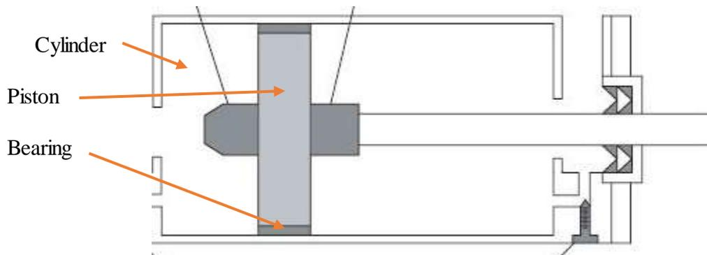
Figure 10: Schematic of Typical Fluid Actuator<sup>14</sup>
